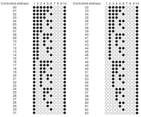
**Note: 1)** once DALI device type and address control mode are selected, please then select the DALI address (00-63 selectable) to be controlled on DALI line by dial switches.
