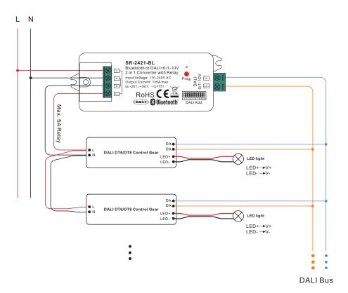
Note: 1) Max. 50mA DALI bus PS output to supply control current to up to 25 control gears.
